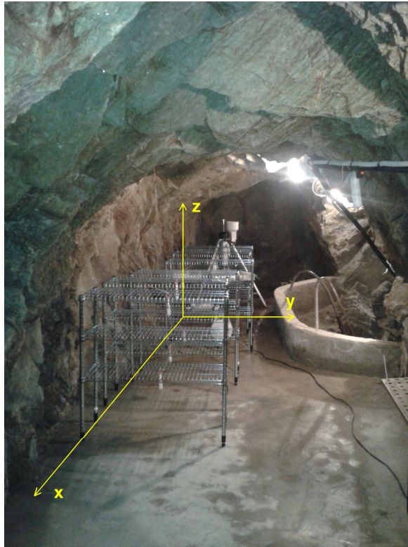
Figure 3.1. The shelves where the dosimeters were placed during the intercomparison: the Cartesian reference system allows to trace the position of the dosimeters sets.
