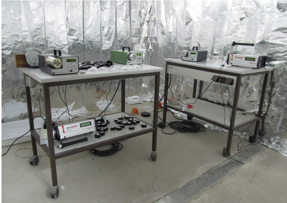
Figure 2.5. Calibration of the monitors in the “radon walkable chamber” (SRP).
